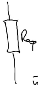
$$R_{eq} = \frac{R_1 \cdot R_2}{R_1 + R_2}$$
